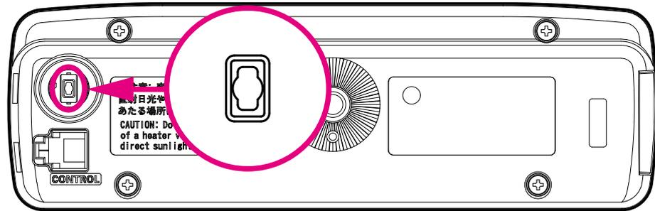
Connect the SCU-20 cable to the MAIN RF body rear mini-Din connector (the mini-Din connector notch should be upward), and then connect it to the USB on the PC.
