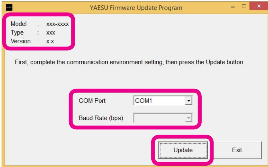
Press the Update button to display the below screen. The procedures required to prepare the transceiver to receive the firmware update are listed, carry out the respective tasks as follows
