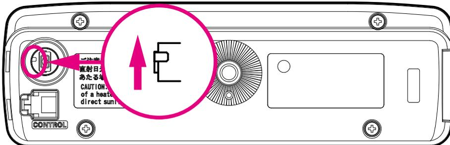
Replace the rubber cap on the panel back.
