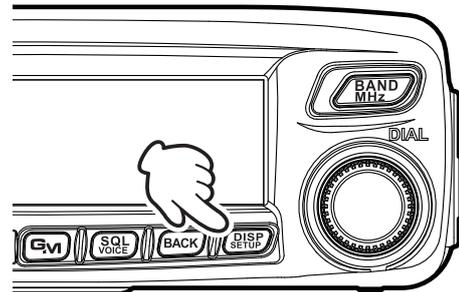
Rotate the DIAL to select [1 FACTORY RESET], then press the
