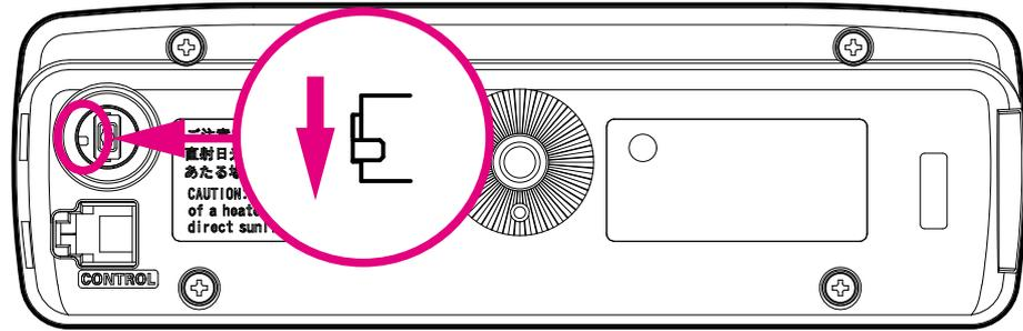
Push the RESET-SW button down. The display will flash one time. (We recommend using a small plastic screw driver or equivalent; avoid using a metal tool because the radio is turned ON).
