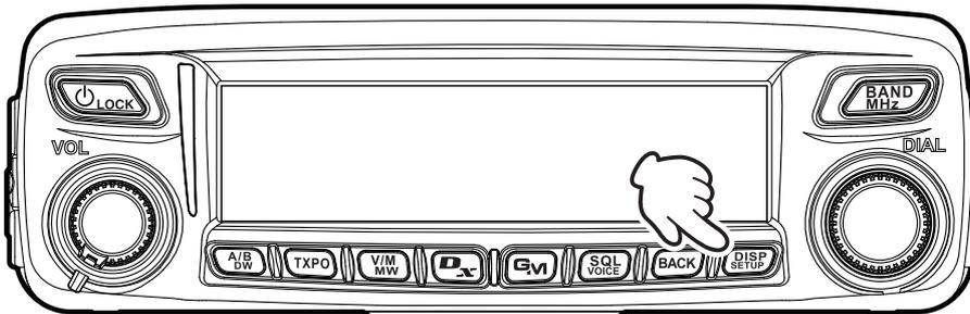
The LCD screen will be blank and a “pepo” signal will sound several times, the Control Panel will enter the write mode.
