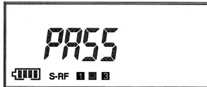
**NOTE** : The memory channels passed from scanning process is automatically recovered when the radio is switched off and on again.
