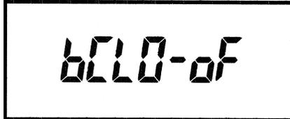
If you press the "▲ or ▼" button in this setting mode, Busy Channel Lock Out will toggle and the changed contents will appear on the LCD.
