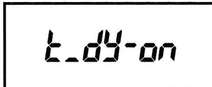
If you press the "▲ or ▼" button in this setting mode, TX delay option will toggle and the changed contents will appear on the LCD.
