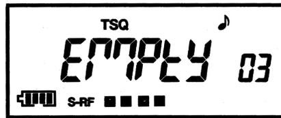
If only one channel remains due to the passing of channels from the scanning process, the process will stop and "EMPTY" message will appear on the LCD.
