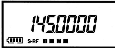
**NOTE :** If you have selected a frequency which is above or below the frequency range allowed, the unit will automatically go to the nearest value.
