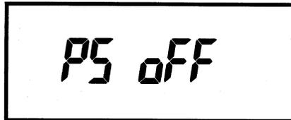
If you press the "▲" or "▼" button in this setting mode, power save On/Off will toggle on the LCD.
