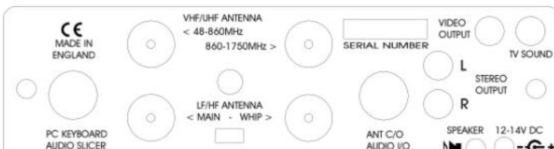
socket or a VHF/UHF aerial into the upper N-Type sockets. Connect the power supply to the receiver and plug it into a suitable mains supply. (See chapter 2 for more information on power supplies and aerials).
